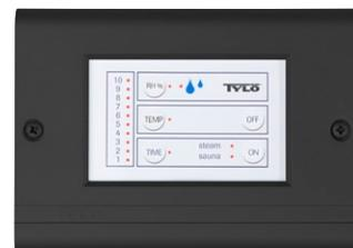
The control panel may be placed inside the sauna room for easy access (max. 1 metre above floor level) or outside the sauna room. The control panel can also be placed on either side of the sauna heater itself (Combi 6 RC and 8 RC).
